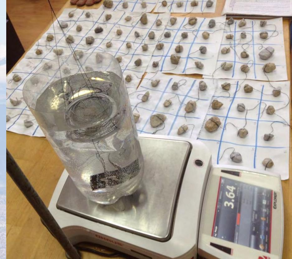
$$|\vec{E}| = |\vec{P}| = \text{mass}_{\text{fluid}} * g = (\rho_{\text{fluid}} * \text{volume}_{\text{fluid}}) * g$$
