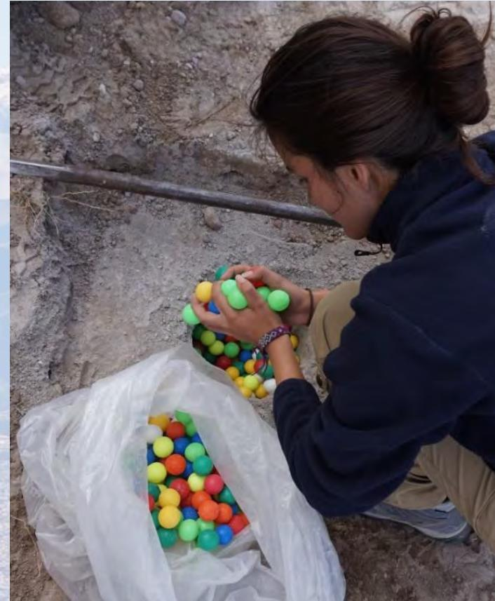
$$volume_{deposit} = 23,593 * (\# \text{ plastic balls}) - 0,7497 \quad (cm^3)$$
